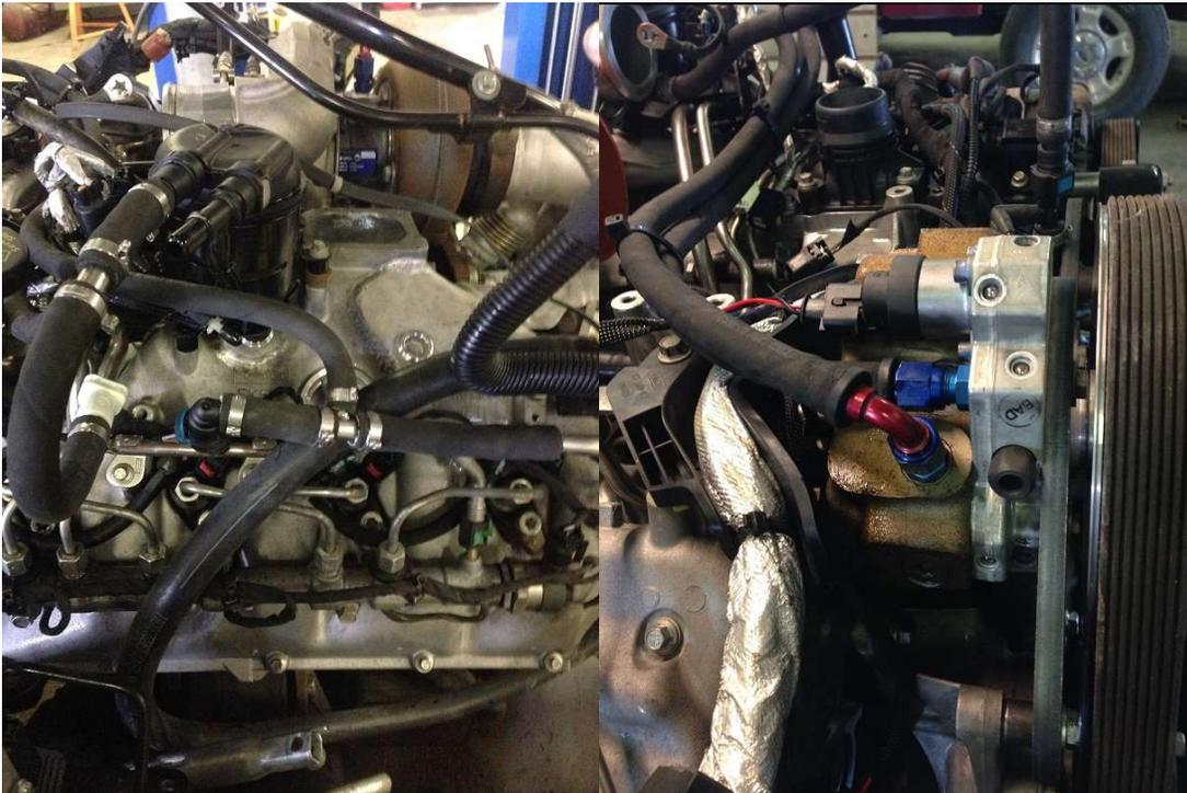
10. Check all fittings and hoses for leaks with key cycled and fuel pump on. Check all bolts and hardware for tightness. Visually inspect belt alignment. Make sure all tools and parts are free and away from moving parts in belt line. Start truck and check for operation.
