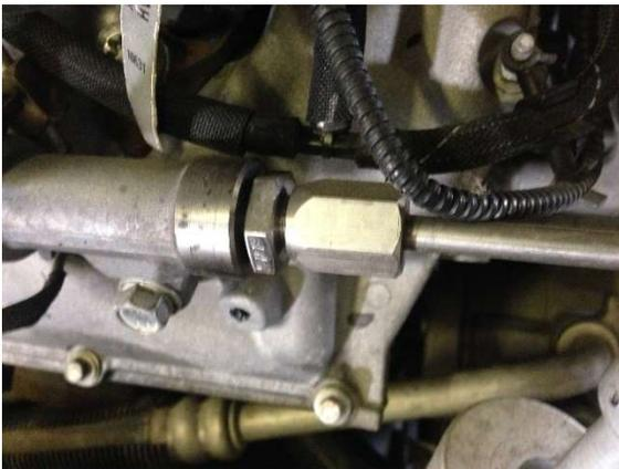
5. Replace with new supplied rail adapter fitting. Install high pressure line
