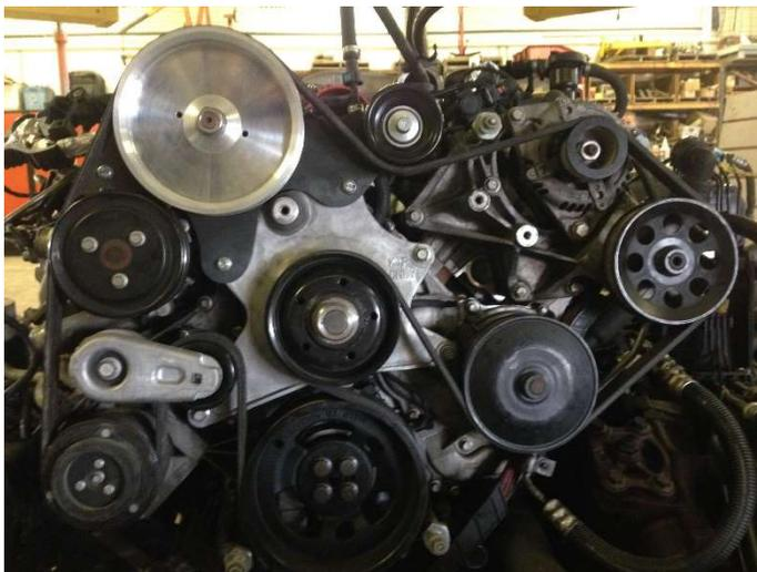
The single sided belt trucks will use the supplied new belt. The idler pulley will be reinstalled into the front cover in position shown.
