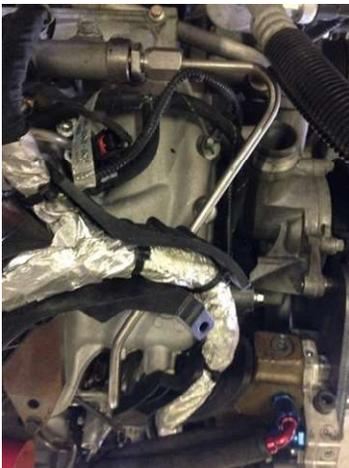
6. Unplug factory hpfp harness and remove yellow center plug "key". Plug new T-harness into factory pump and engine wiring harness, then plug into cp3 pump.
