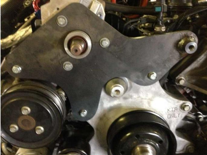
4. Remove passenger side rail end plug with 12pt torx socket.
