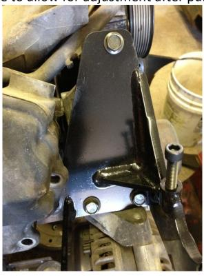
3. Remove old idler pulley and install new one included in kit
