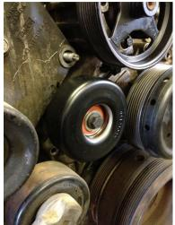
4. Mount pump to bracket. Using allen bolts. The battery box will have to be clearanced. Using the pump pulley in the kit mark out where they will intersect and trim battery box to suit.
