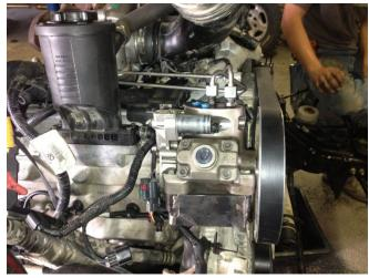
6. After pump is mounted and belt ran you will need to install the hp fuel lines. You will have to unbolt the heat shield from the
